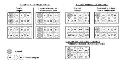
For reasons of simplicity the procedure described below is for a test on 3 water samples with 2 replicates and 1 hour exposure.
