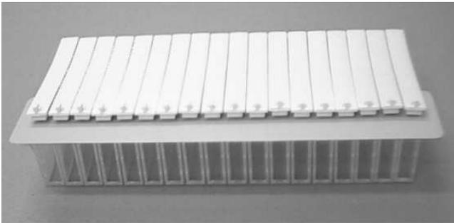
2. Put the holding tray for 3 days in an incubator or in a temperature controlled room, with a constant uniform illumination supplied by cool white fluorescent lamps; make sure that the illumination is 10000 lux for sideway illumination or 3000-4000 lux for bottom illumination.
