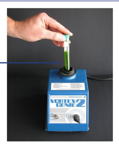
SHAKE THE TUBE ON A VORTEX UNTIL THE MATRIX IN WHICH THE ALGAE ARE IMMOBILISED IS TOTALLY DISSOLVED AND THE ALGAE ARE SET FREE
