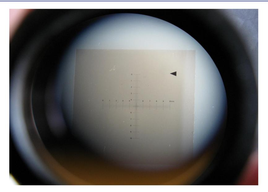
PUT THE MICROMETER SLIP ON THE GLASS STAGE OF THE DISSECTION MICROSCOPE, IN THE CENTRE OF THE VISUAL FIELD
