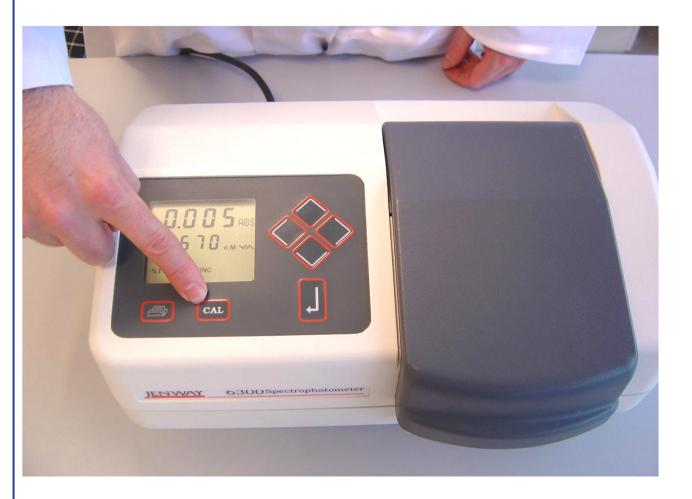
ZERO-CALIBRATE THE SPECTROPHOTOMETER PRIOR TO THE DAILY MEASUREMENT OF THE OD IN THE LONG CELLS,
