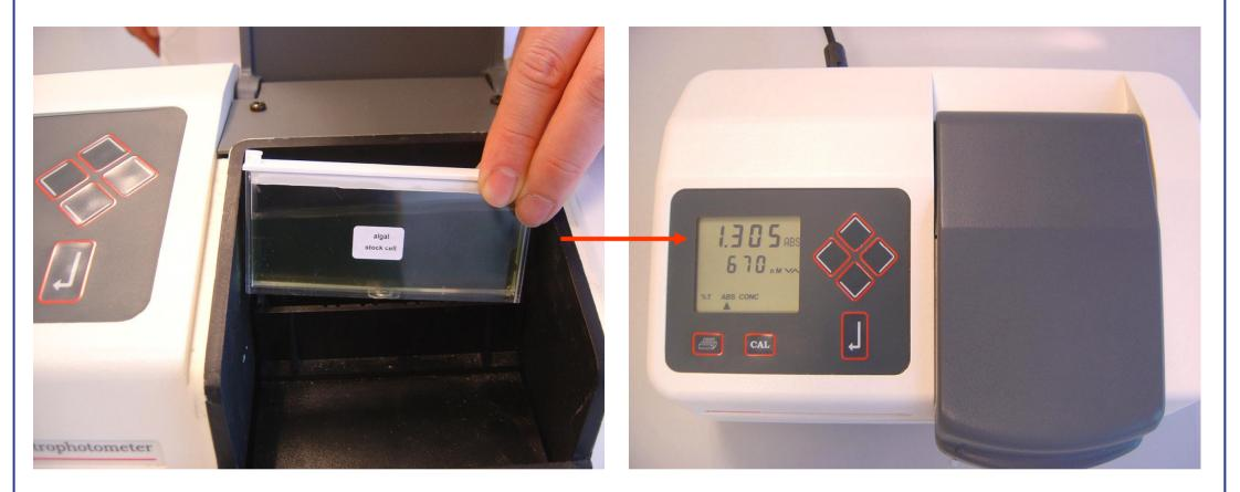
PUT THE ALGAL STOCK CELL IN THE SPECTROPHOTOMETER AND READ THE OPTICAL DENSITY (**OD1**) AFTER 10 SECONDS
