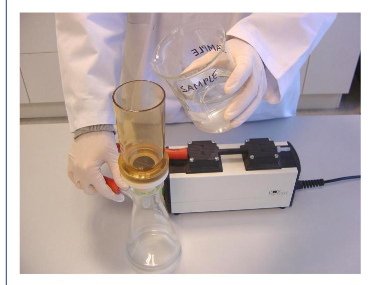
TO ELIMINATE TURBIDITY, SAMPLES MUST BE FILTERED BEFORE TESTING (e.g. over a membrane filter of 0.45 μm),
