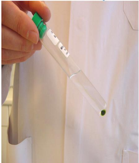
CENTRIFUGE THE TUBE FOR 10 MINUTES AT 3000 RPM IN A CONVENTIONAL LAB CENTRIFUGE
